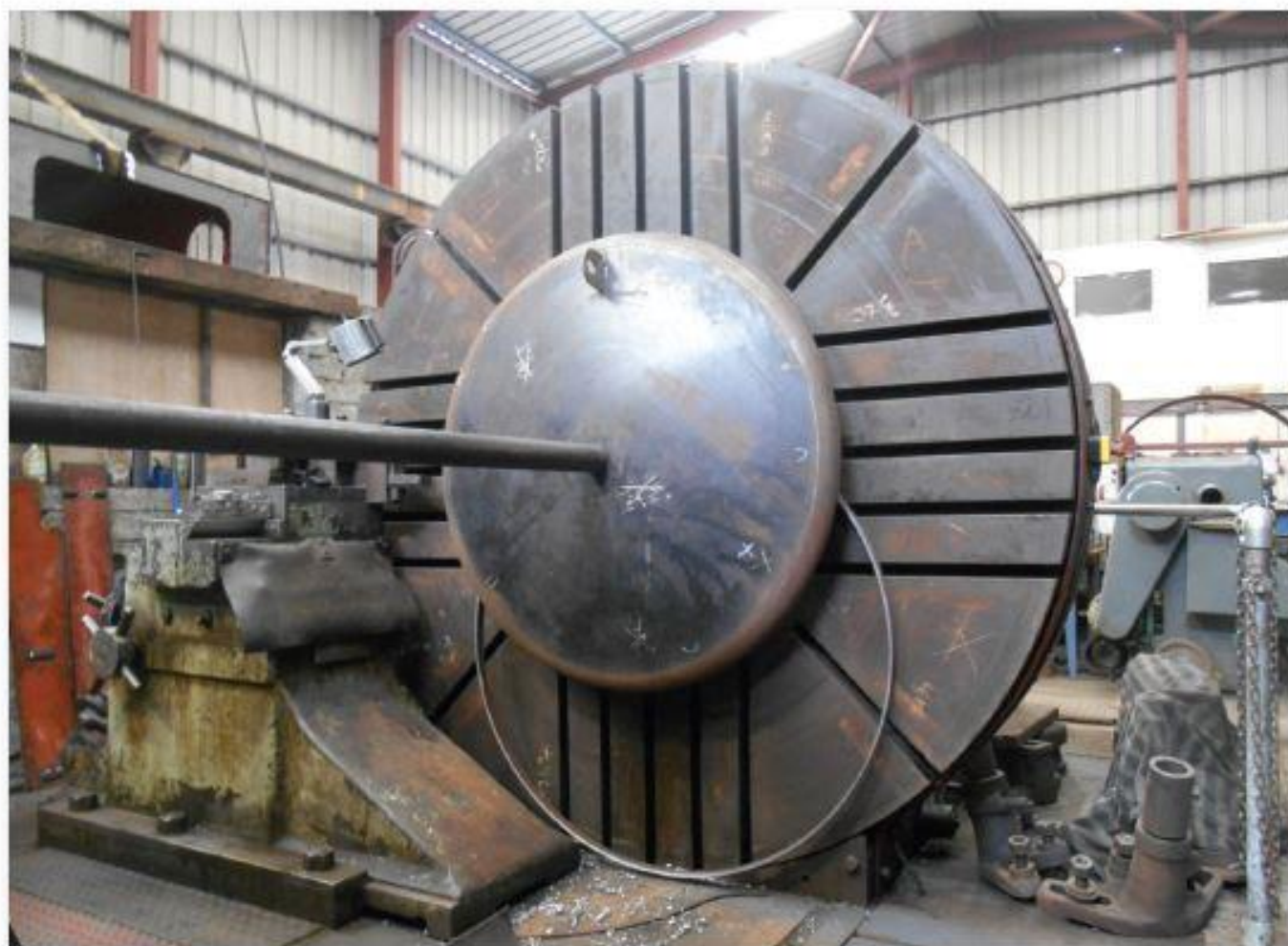
Smokebox doors can be made from 'dished ends' (ie the end of a cylindrical silo) by the wheel lathe, which in many regards would be better named a 'round thing lathe'. Braced by the bar against the opposite centre of the lathe on 6th June, the dished end has been spun in order to shave off a ring of surplus material and bring No.105's door down to the correct size. (Photo: Editor)
