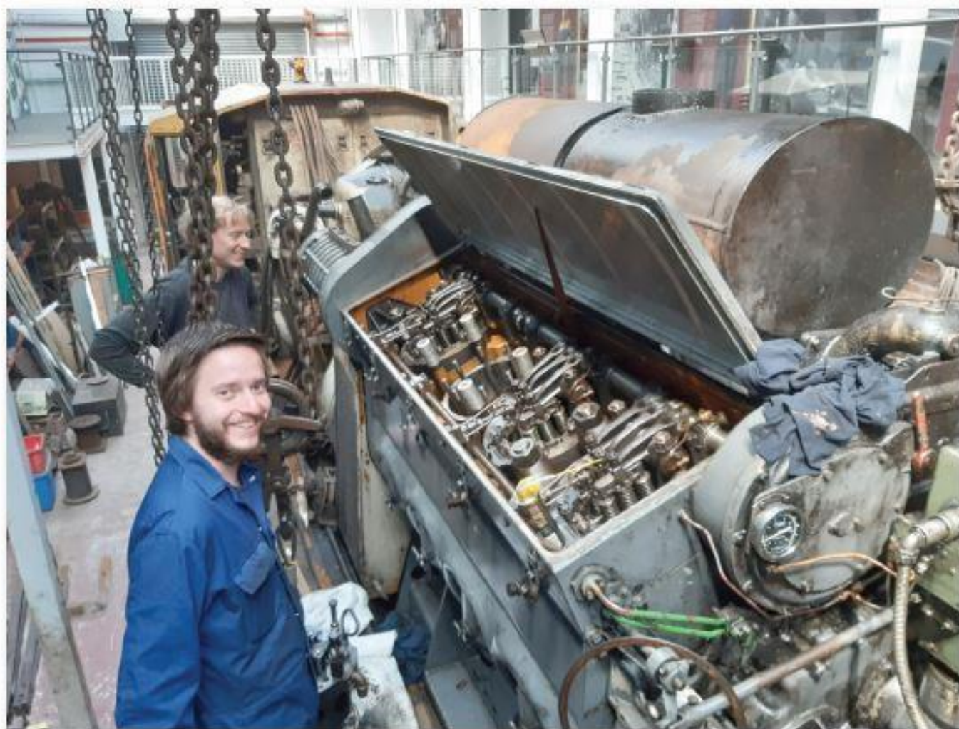
Phillip Newell and Alan McKnight (foreground) rebuilding B142's power assembly head 3, the hole for which can be seen in the engine between Nos. 1 and 5 (of 8), 25th April. (Photo: J Friel)
