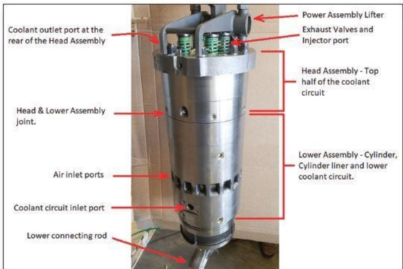
A cleaned up power assembly from B142, with parts labelled.
