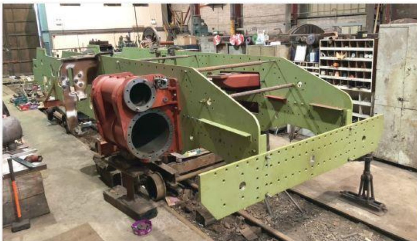
No.105 steadily began to take shape in the workshop throughout 2021. It has gained its bufferbeam (by Portillo!), cylinders and motion brackets. (Photo: N Lawrence)
