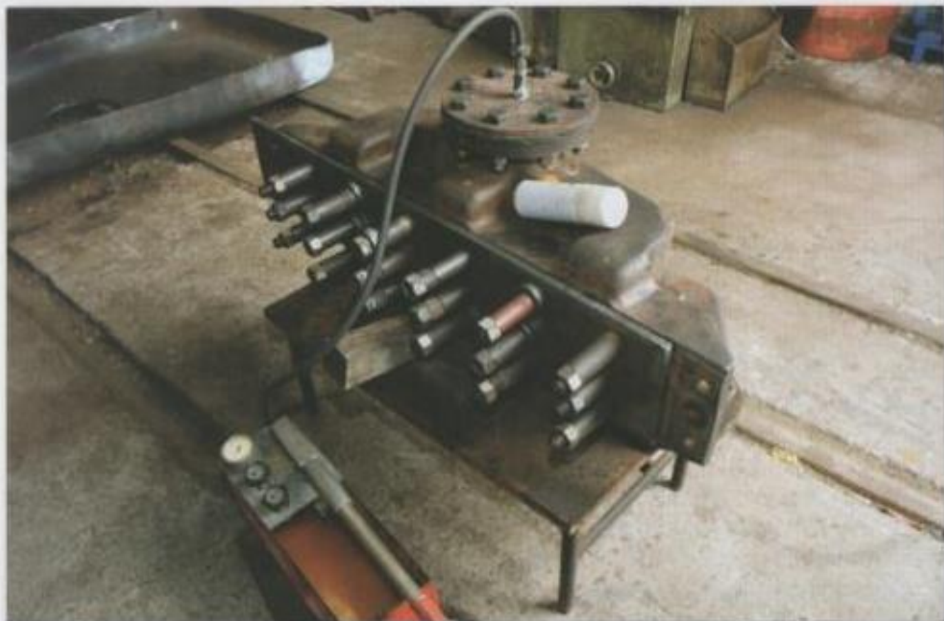
No.171's superheater header, normally found in the top of the smokebox, set up for hydraulic pressure testing, 12th July. (Photo: B Hill)
