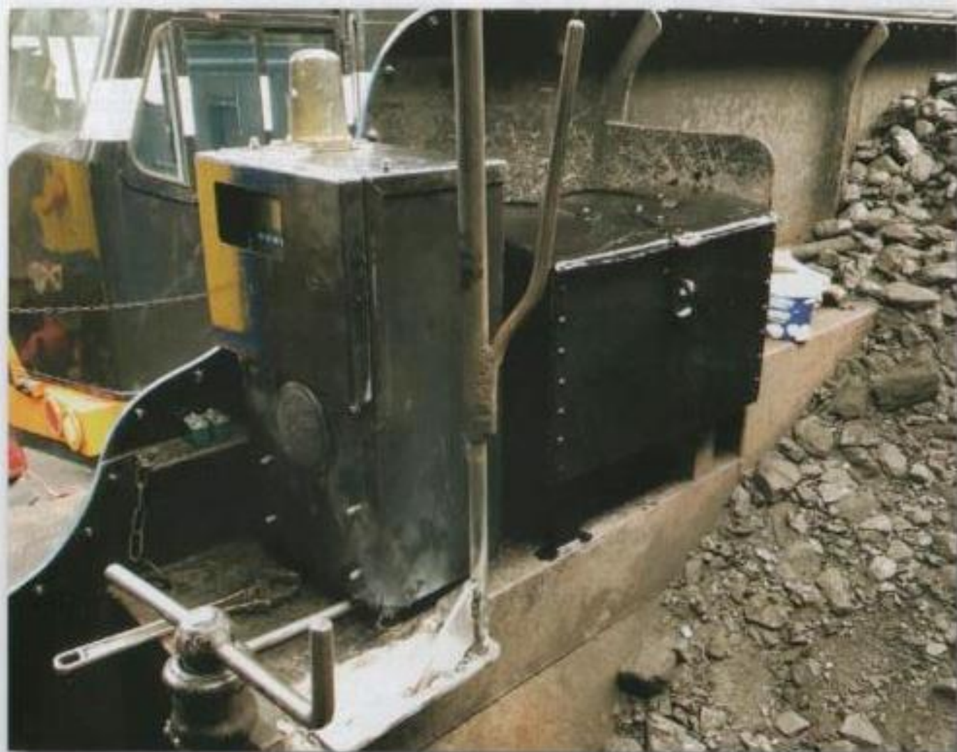
No.85's new Irish Rail train radio, 21st July. It can be seen that as technology increases, the toolbox / crew belongings space on our locomotives continues to decline. (Photo: N Lawrence)
