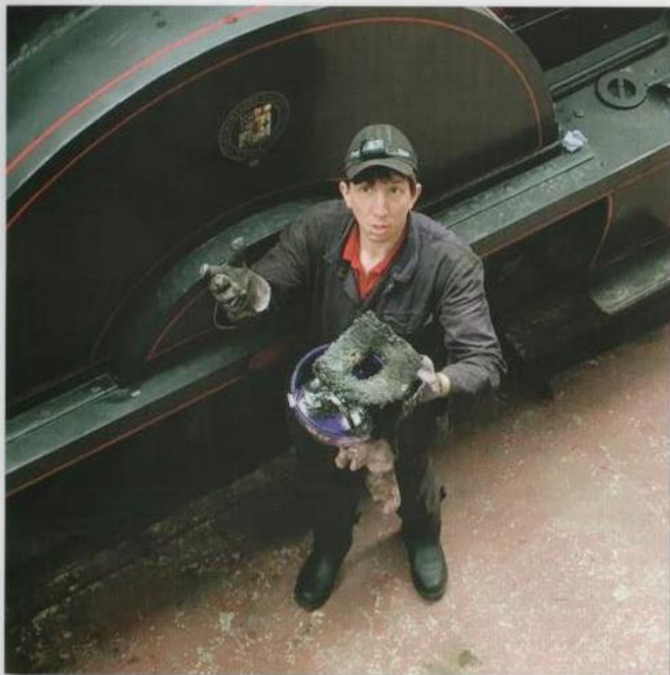
The Editor explains the innards of an axlebox to visitors on the upper floor of the museum during 131 spongepad replacement on 19th May. (Photo: R Morton)
