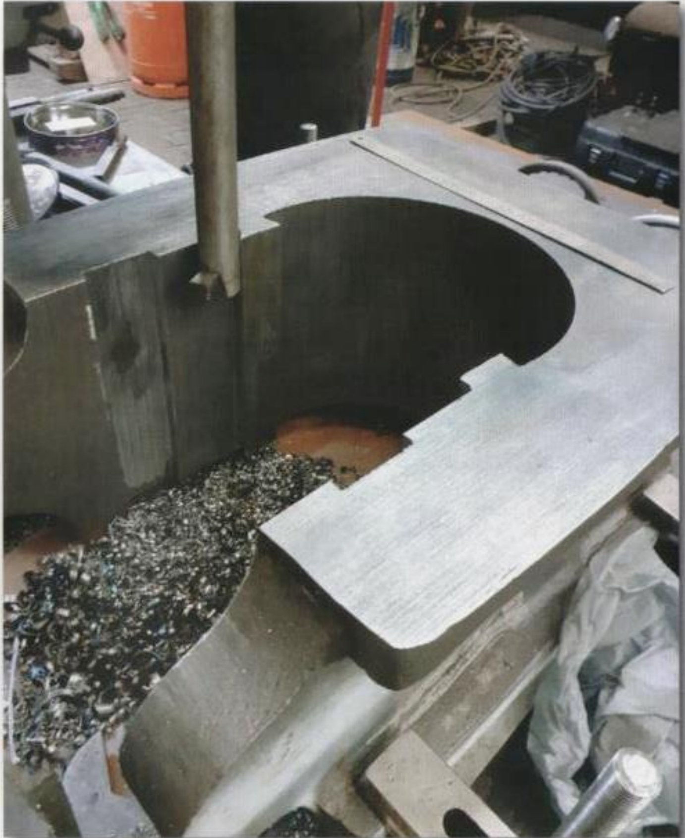
Slotting the groove for the sponge box in a mogul axlebox, 19th May.
