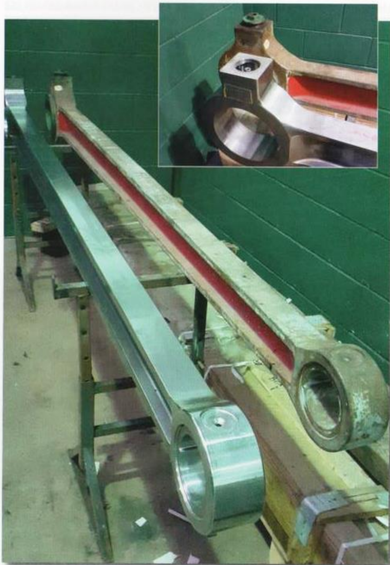
New and old con rods, and a close up of their big ends, Feb 2023.
