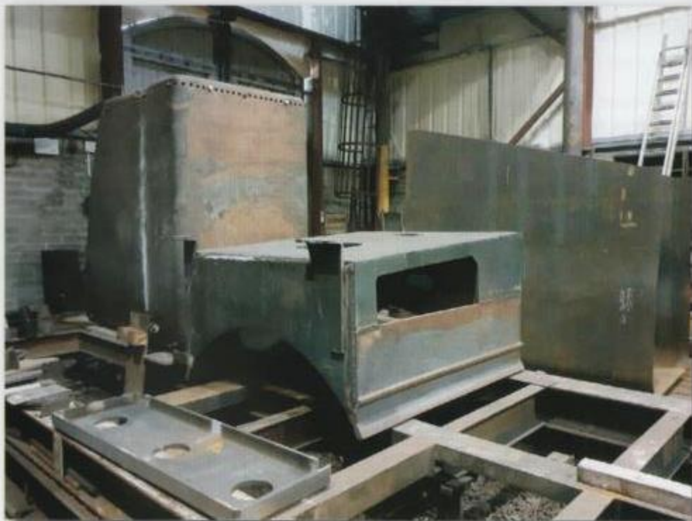
Smokebox saddle, G8.24 inner firebox and outer wrapper, Feb 2023.
