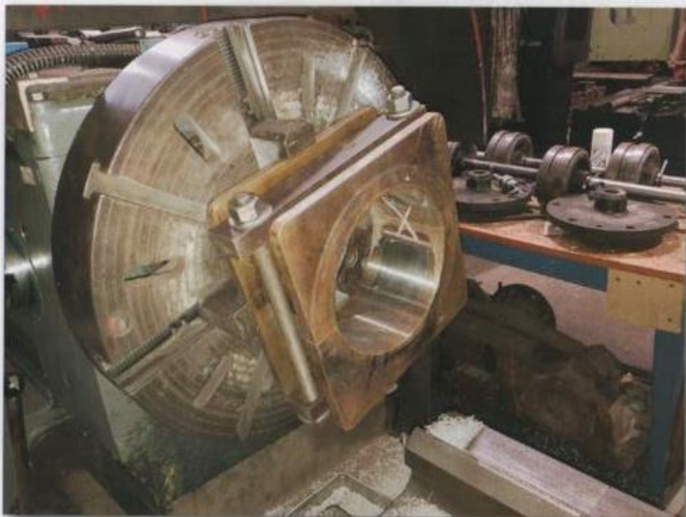
No.85's centre (high pressure) big end bearing gets machined (yet again) following re-metalling at Whitehead on 6th November. This again failing in December, new brasses to original, unworn design size have been ordered and delivered for 2023.
