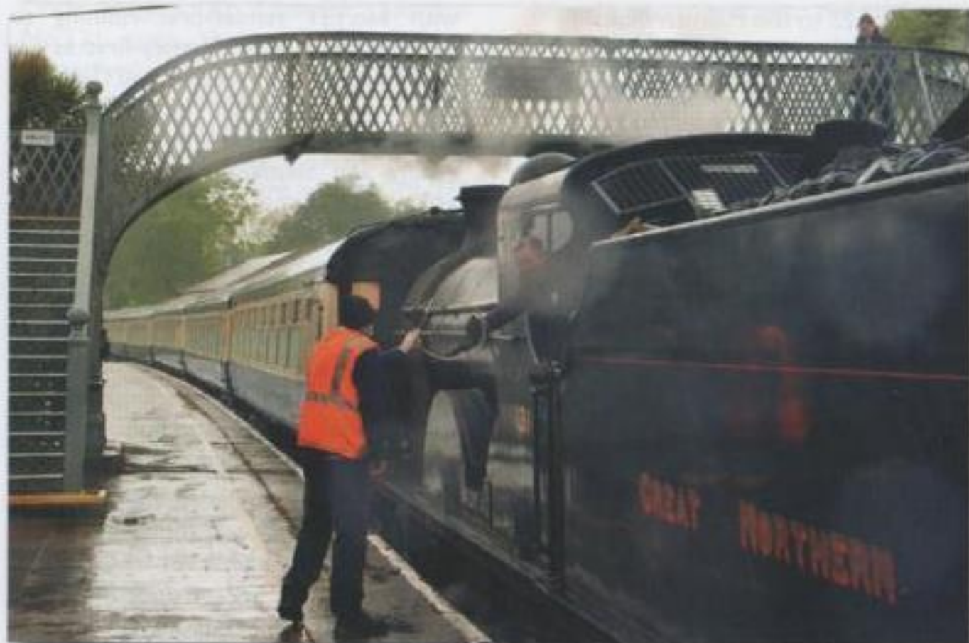
The signalman at Carrick-on-Suir hands Ken Fox on No. 131 the staff for Waterford West, on a wet 09th May. The staff from Clonmel lies where Ken dropped it off, by the bottom of the footbridge steps.
