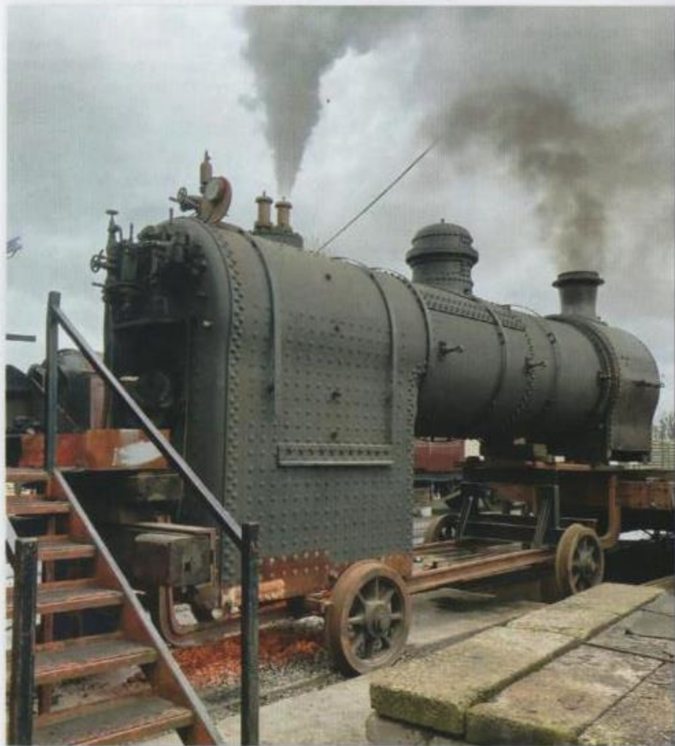
No.171's boiler blows off on 20th December, as it undergoes its out-of-frames boiler inspection which it passed that day. (Photo: Editor)
