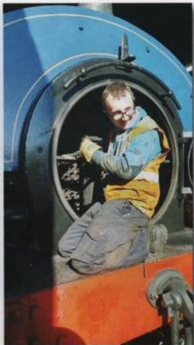
Sam Hall cleans out boiler tubes on 3BG, 15th October. (Photo: Editor)
