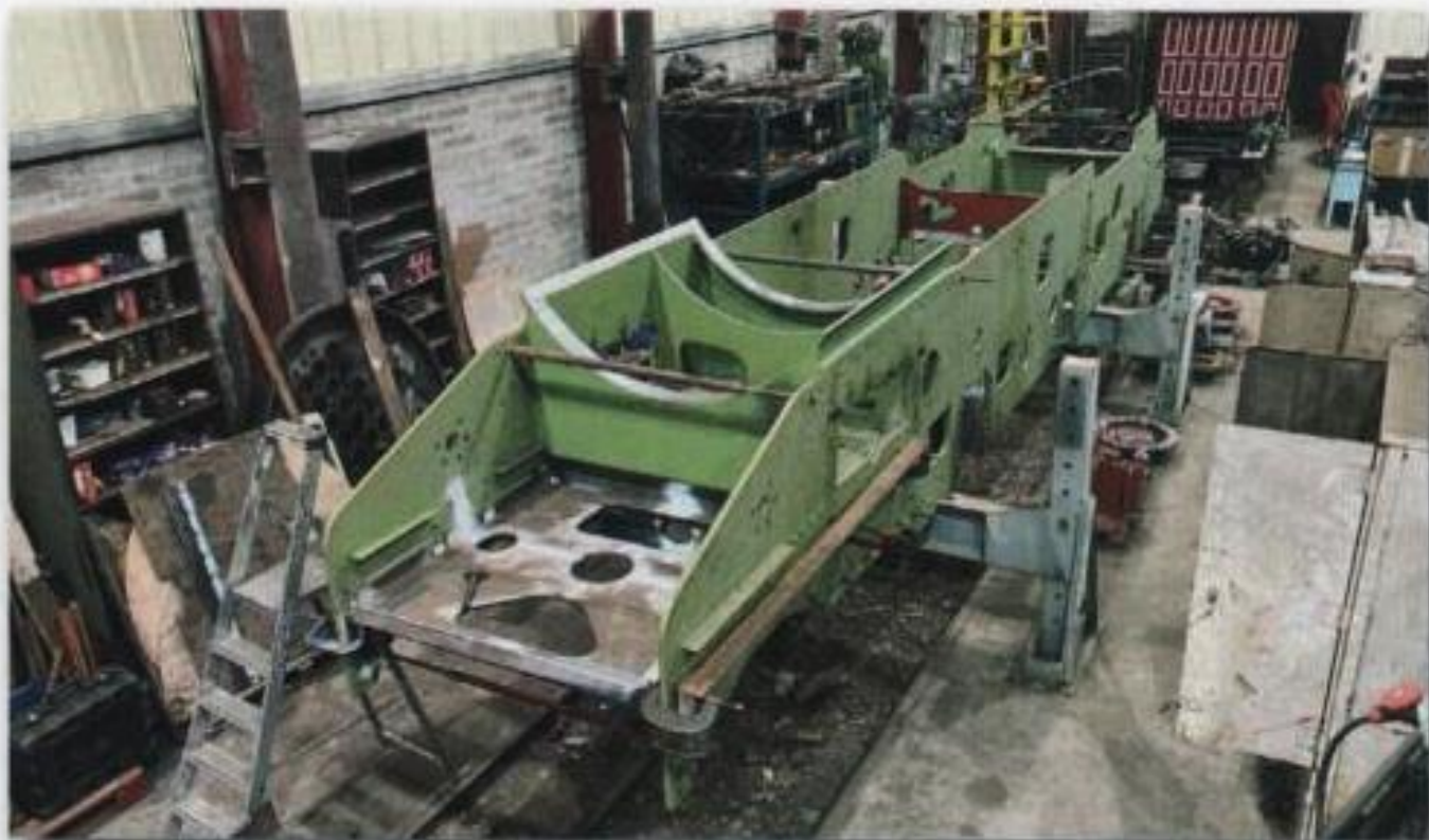
Frames showing flanged plates, stretchers and smokebox saddle, 05th November. (Photo: N Lawrence)
