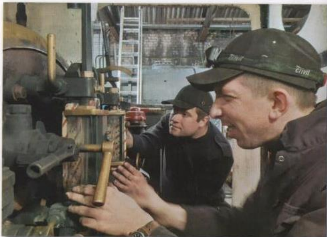
The Editor and Adam Lohoff refit pieces to 3BG's gauge glass assemblies prior to her annual boiler inspection, 17th November. (Photo: JJ Friel)
