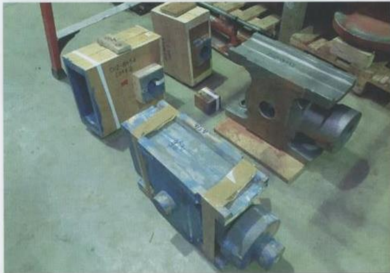
The crosshead pattern equipment and a new crosshead casting, 31st December
